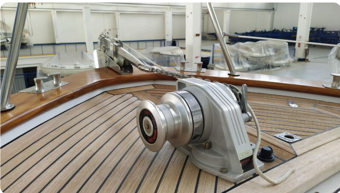
Apreamare 9 Open - Windlass Detail
