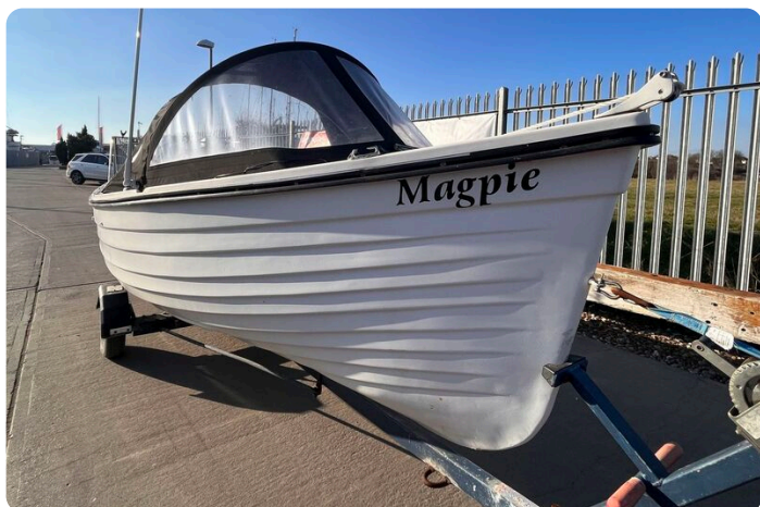
Fisherman 17 clinker boat - clinker style hull
