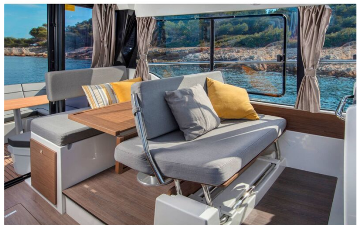
Jeanneau Merry Fisher 1095 - table folds and forward seat converts to co-pilot seat
