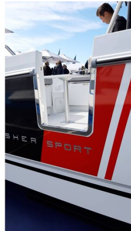
Jeanneau Merry Fisher 795 Sport - Series 2 - cockpit side gate for easy access to pontoon
